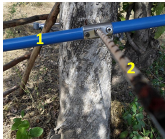
Fig. 4 Wood sample obtained from increment borer. CHABI, October 2014. 1 Increment borer, 2 wood sample
