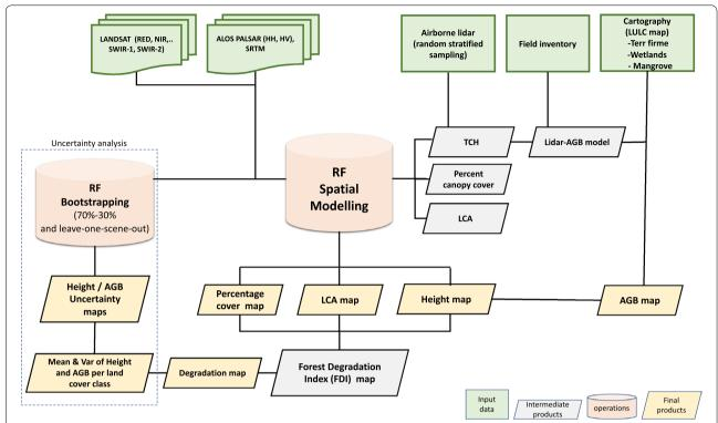
**Fig. 1** Flowchart showing the steps leading to the production of an AGB map. Data inputs are shown in green, intermediate products are shown in grey, while operations are shown in pink and final products in yellow. Operations and products related to the uncertainty analysis are shown in a dashed box. AGB aboveground biomass, TCH mean top canopy height, LCA large trees canopy area
