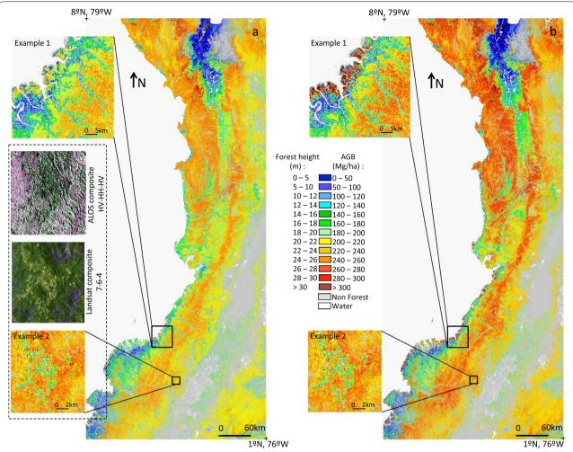
Fig. 4 Height map (a) and AGB map (b). Example 1 shows how mangrove forest stands out in the AGB map because of its higher wood density. Example 2 displays the signature of fragmentation, as seen in ALOS and Landsat
